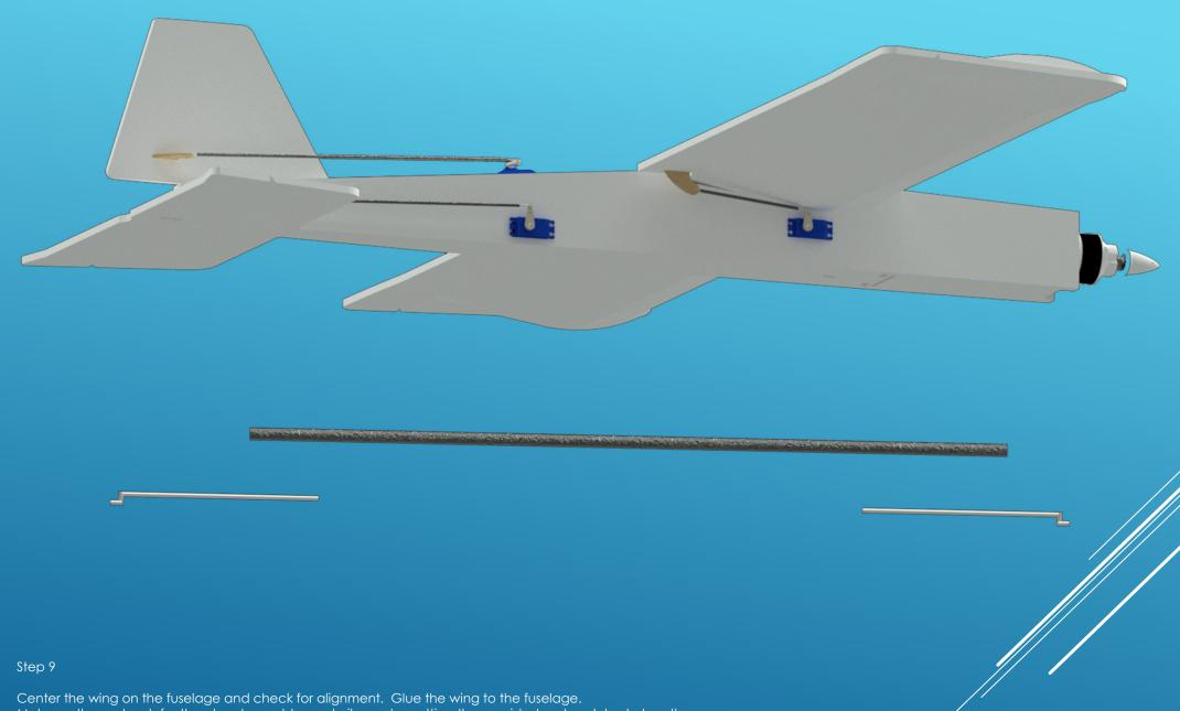
Center the wing on the fuselage and check for alignment. Glue the wing to the fuselage.
